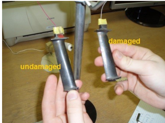
Fig. 14. Turbine blades (damaged and undamaged) for laboratory experiments.
