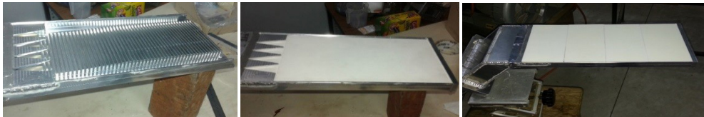
Fig. 1. Comb applicator (left) without covering with ceramic plates. Ceramic applicator (middle) without covering by ceramic plates. Comb and ceramic applicators view (right) covered by ceramic plates (3x84x146 mm - 4pc).
