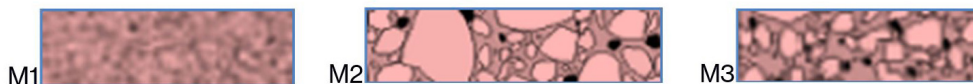
Figure 5: Excessively fine M1 (unsuitable), discontinue M2 (less suitable) and Well graded M3 (more suitable combination).
