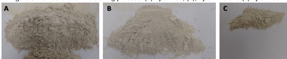
Figure 9: Powders after the sieving process: (a) Tyler 200, (b), Tyler 270 and (c) Tyler 400.
