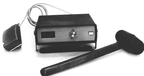
Fig. 22. General view of the device for express monitoring of air pressure in tires.
