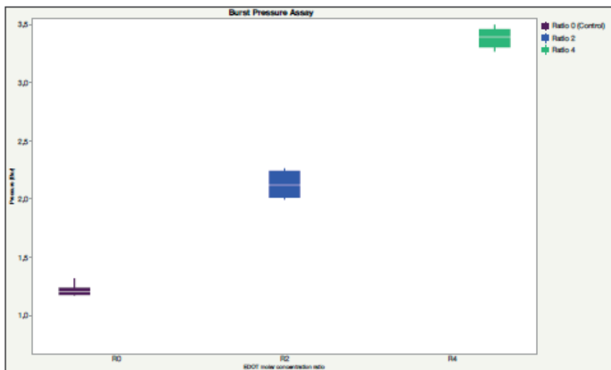
Figure 6. Burst pressure of TEBVs with different APS:EDOT ratios.
