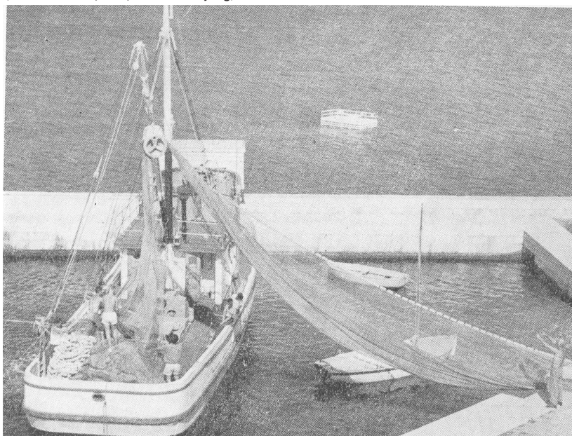
Figure 4. Research vessel PREDVODNIK of Institute of Oceanography and Fisheries with Puratić-block and purse-seine net (From: Morović, 1971; Foto: M. Alajbeg).
