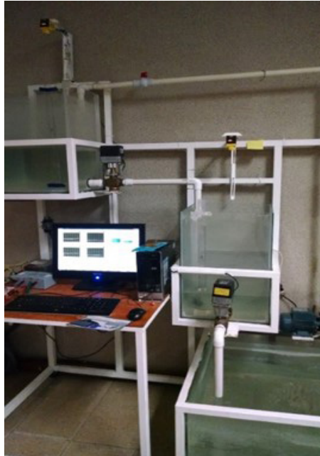
Figure 1. Schematic diagram of the liquid level system.
