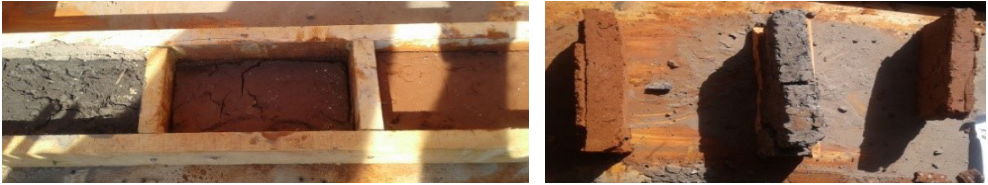
Photographs 3 and 4: Solar drying in molds and outside molds on edge:
