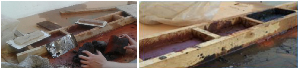
Photographs: 1 and 2: Kneaded and compacted materials in molds.
